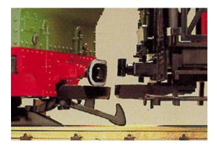
LGB "hook and loop" couplers are engineered for easy, reliable operation, even on uneven track sections.
