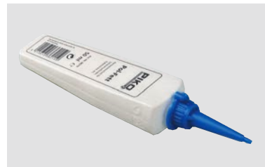
36215 Conductive Paste, 50 ml Helps keep out corrosion-causing moisture - especially important for garden railroads. Use in rail joiners, in RailClamps, on electrical terminals such as switch machines and even on electrical contacts of locos and lighted cars.
