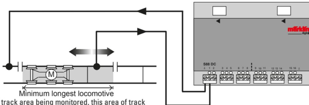
If there is a signal within the track area being monitored, this area of track without current can be included in the monitoring by means of a resistor (1.5 kilo ohms).
