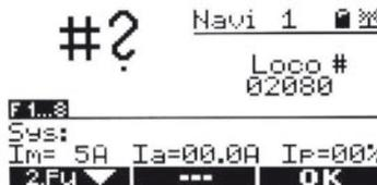
In Driving Mode the selected locomotive address is now available. If the locomotive address that is entered is not defined, the result is a first vehicle operation for new locomotives with undefined locomotive characteristics.
