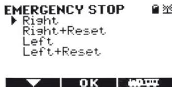
Use this menu item to select the preferred Emergency Stop Mode, for example, depending upon whether you are left- or right-handed. You define the key to be used to initiate an EMERGENCY STOP using LEFT or RIGHT. You can reinitiate an EMERGENCY STOP using the second STOP key. The RESET option allows the transmission of an additional STOP command. All locomotives are stopped however the voltage is not switched off
