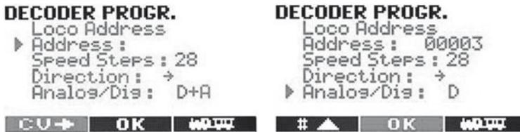
This is where you can read and program in the locomotive address for your locomotive. The address can be selected from 1-1-10239. The Navigator automatically calculates the appropriate programming values for CV 1, 17 and 18+29. In addition, you can also indicate whether the decoder should be operated with 14 or 28 speed steps or set the driving direction and block the analog operation.
