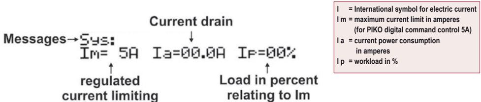
The menu bar displays the current configuration of the 3 key **M1**, **M2**, **M3**.
