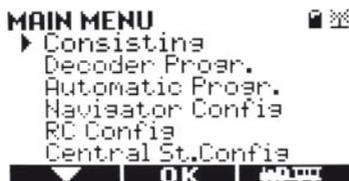
The principal underlying the menus is universal.  $M1$  is used for navigation,  $M2$  is used to confirm a selection and  $M3$  returns you to vehicle operation. You can change the selection using  $M1$  until you reach the desired menu item and then conform your selection using  $M2$ .
