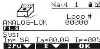
**NOTE:** A high frequency whistle generated by analog locomotives on a digital track is caused by a particular form of digital tension. Extended operation is not recommended. A change of lights is generally not possible. (Refer to the manufacturer's instructions.)
