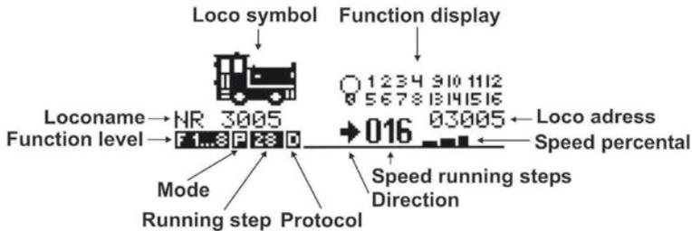
The secondary function field displays the following information when activated:
