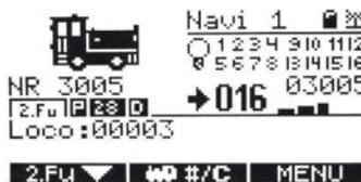
If the locomotive address has been correctly selected, the data associated with the locomotive will be shown in the display. Those data include: locomotive address, locomotive name (if assigned), light, functions 1 through 8 and of course the direction of travel and the speed step.
