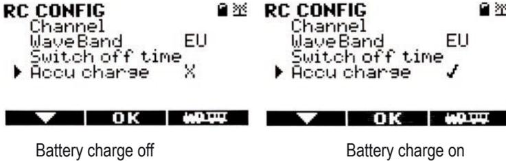
**IMPORTANT NOTE: only activate the charge function on the Navigator if rechargeable batteries have been installed. Non-rechargeable batteries may not be recharged under any circumstances. This will destroy the battery. There is a risk of explosion!**
