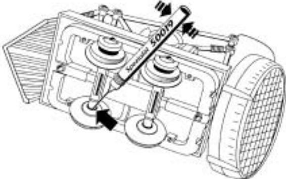
Fig 1. Lubricating the wheels 1
