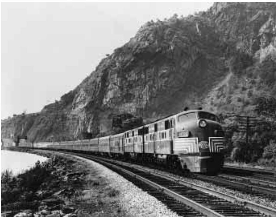
The "new" 20th Century Limited at Breakneck Mountain on the Hudson River. In the 1940s and 1950s, the train consisted of 16 cars, pulled by a 4000 hp, double-unit diesel loco. New York Central photo, courtesy of Kalmbach Publishing Co.
